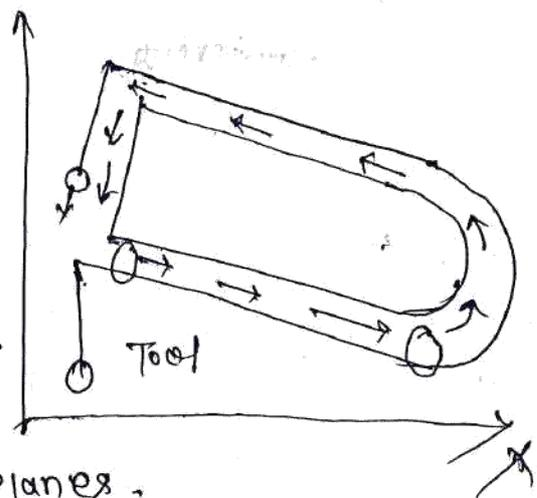
→ Contouring NC M/Cs have a complex circuitry / design which can feed & read information of the tool that are normally programmed with the help of computers. This system is commonly used in milling machines.
