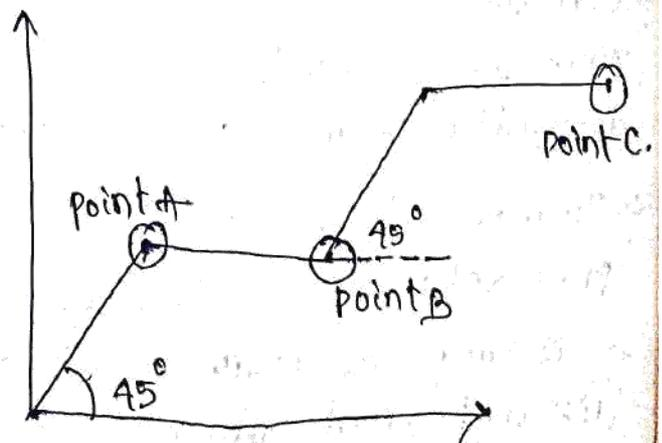
→ In these machines after the drilling M/C is performed the tool is moved to the next location for the operation till the operations are completed.
