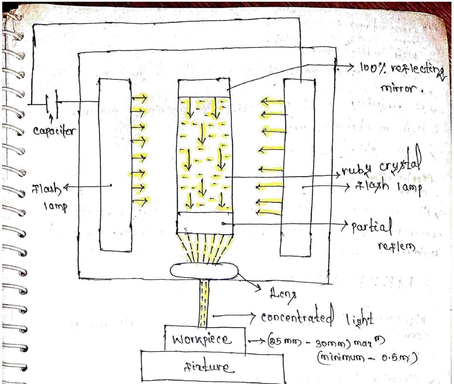
Laser (Light amplification by stimulated emission of radiation)
