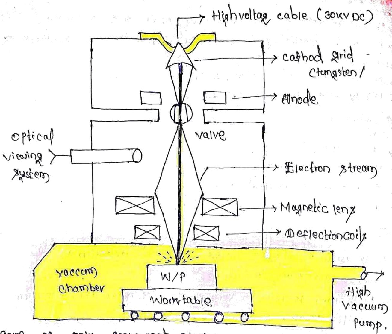
care of only convergent electron passes through it. It absorb all divergent electron & low energy electron. It provide a high quality electron beam.
