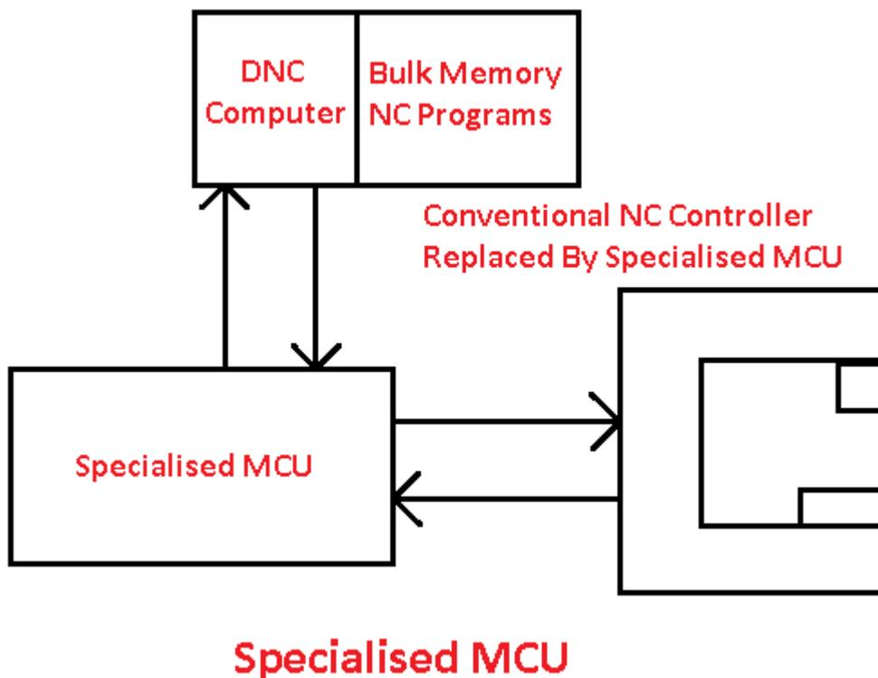
In specialised MCU system, replace the normal controller unit with the special machine control unit. The special control unit is created to help communication between machine tools and computers. The specialised MCU configuration achieves a better balance between the accuracy of interpolation and the faster removal rate of the metal than is usually possible with the BTR system.
