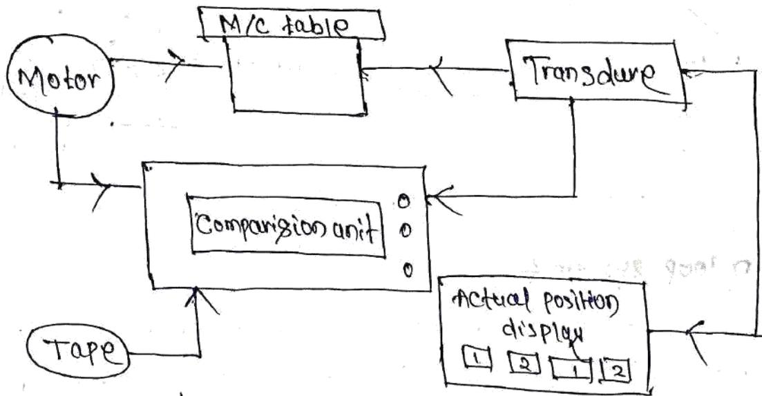
→ In a closed loop system along with the components of an open loop system a feedback unit is added into the electrical circuit.
